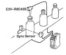
Internal Amp Photoe ectric Switch E37,-R3C43S
